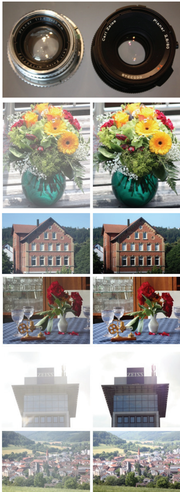
Fig. 18: Left column: Pictures with an uncoated Planar 2.8/80mm; right column: pictures with T*-coated Planar T* 2.8/80mm CFE.
