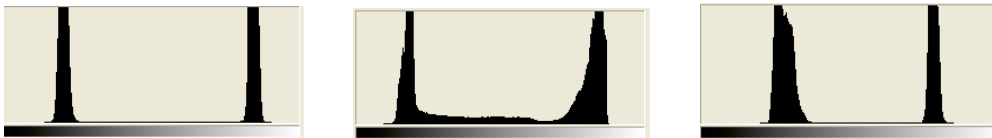
The characteristics of the images above are also illustrated by their histograms: In the picture of the lens with poor micro contrast (middle) the right peak in particular is broadened towards the left, because the white at the edges with glare lights up the areas which are in reality black. The separation of the two peaks on the gray scale is the same as with the good picture on the left, however.
